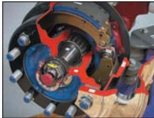
Cutaway View of the Wheel and Brake Assembly of the Steer Axle
