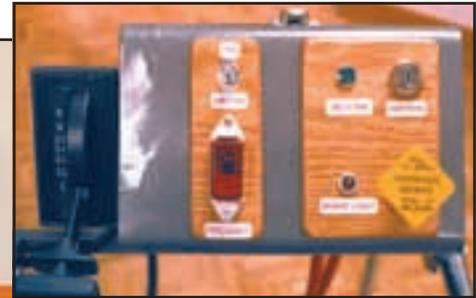
Mock-up of the console shift lever and interlock circuitry that would have prevented the accident
