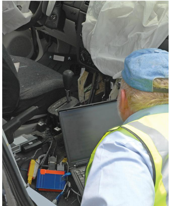
*Data downloaded from the airbag control module is analyzed and then incorporated into the reconstruction.*
