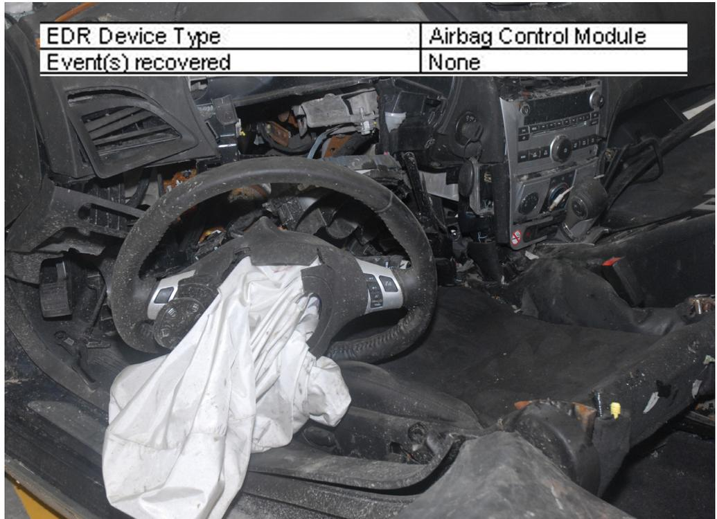
*A deployed airbag is not confirmation that EDR data is present. An electrical power loss can prevent the EDR from recording crash data, and other evidence must be used to reconstruct the crash.*
