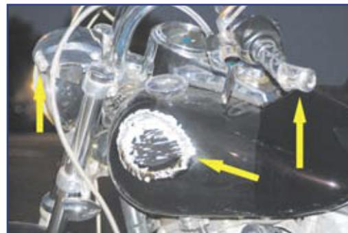
*Contact damage to only the left side of the motorcycle is inconsistent with the witness' testimony that the motorcycle "flipped and tumbled after it was hit."*
