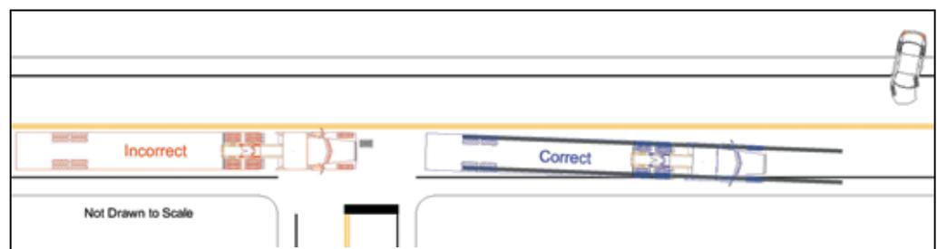
The drawing created by the accident reconstructionist shows the location of the tractor-trailer when the hard brake event data was created, according to each expert. Note that the opposing expert's incorrect location does not match the tire marks on the roadway.
