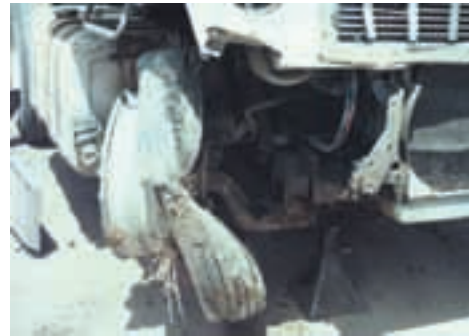
One of the tires on the steer axle of this tractor-trailer had a blow-out. When the tire failed, the driver lost control. The subsequent accident resulted in multiple fatalities.
